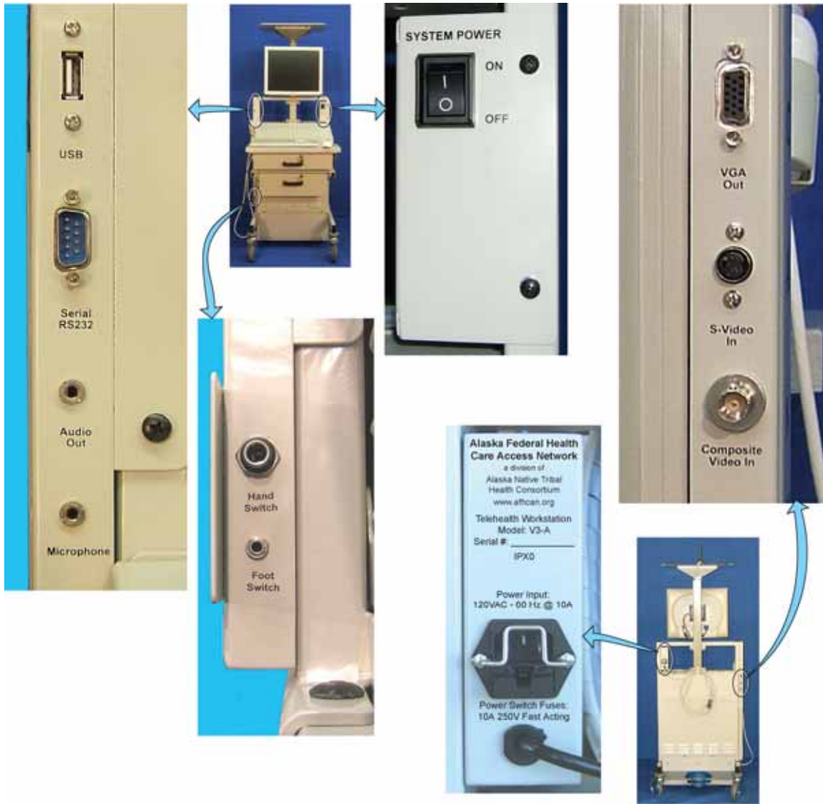
Figure 6 Auxiliary connection points, main power switch, and labels
