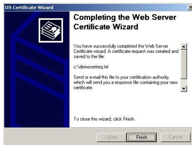
Figure 17 – Completing the Web Server Certificate Wizard
