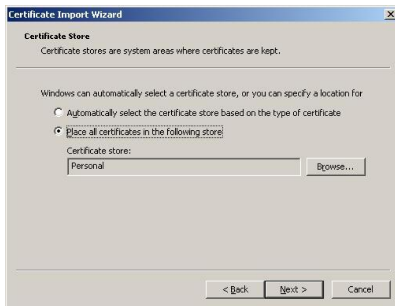
Figure 29 – Placing the Certificate into the Certificate Personal Store
